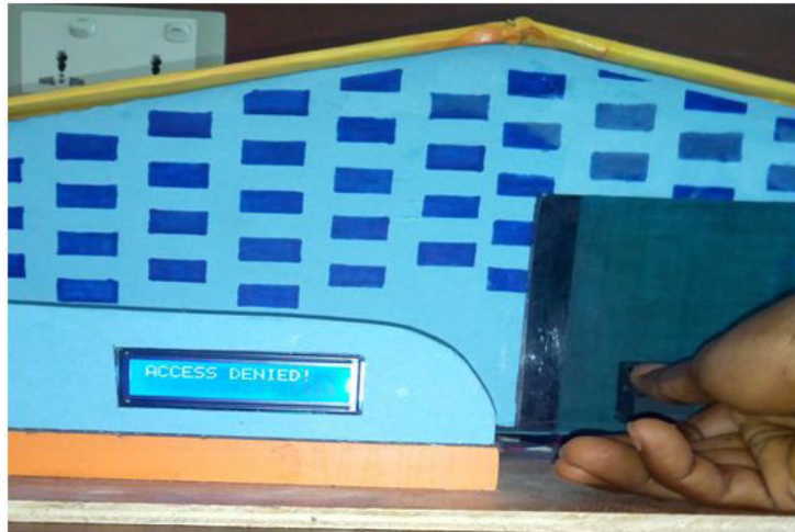
Figure 9: Picture showing access denied to an unrecognized fingerprint
