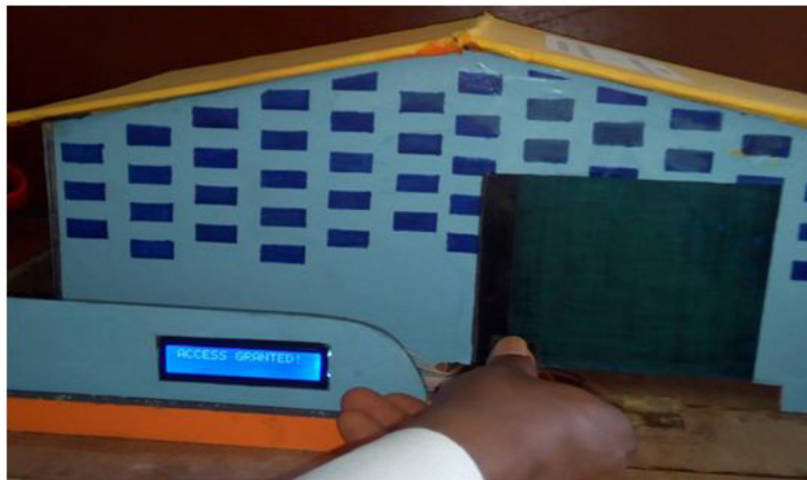
Figure 7: Picture showing access granted to a recognized fingerprint
