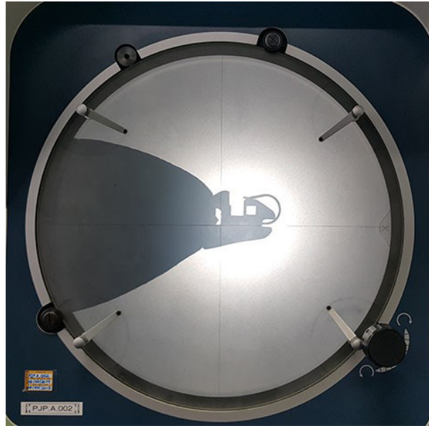
Figure 2: Bracket slot positioning and references axis lines, X (horizontal) and Y (vertical)
