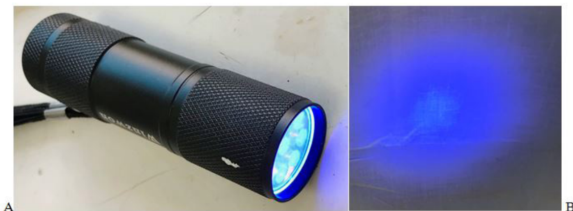
Figure 4: A: Ultraviolet flashlight. B: Fluorescent-stained aerosols on the sheet
