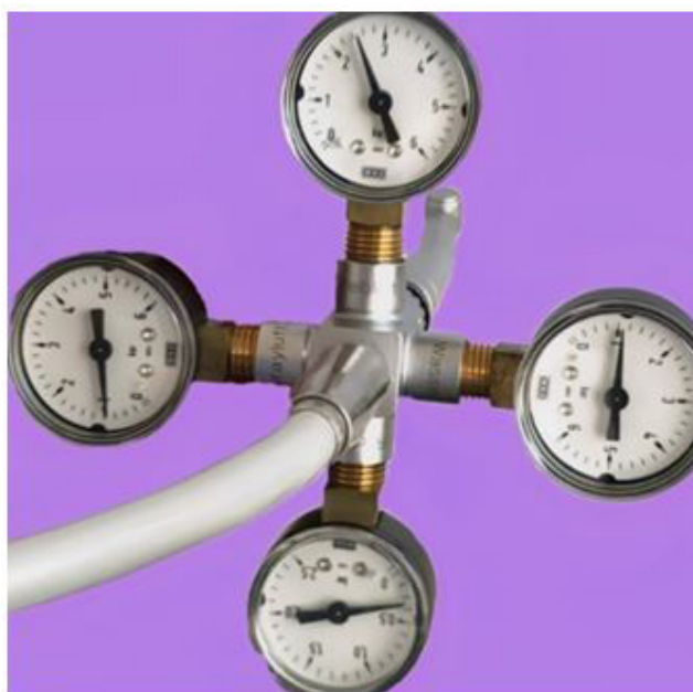
Figure 3: Specific 4-way manometer. Top: air pressure going in the rotor (2.5 bar), Bottom: air pressure going out of the rotor (0.75 bar), Right: air pressure of the cooling spray (set to 1 bar), Left: water pressure of the cooling spray (set to 1 bar)
