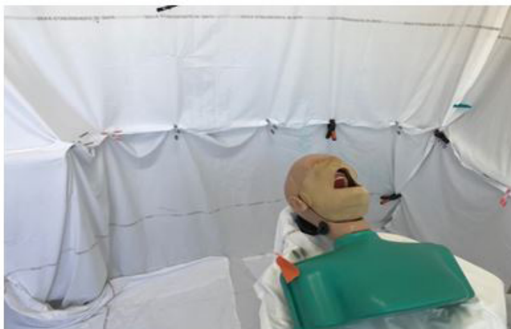
Figure 2: Patient simulator on the dental chair with sheets covering the floor and the partitions
