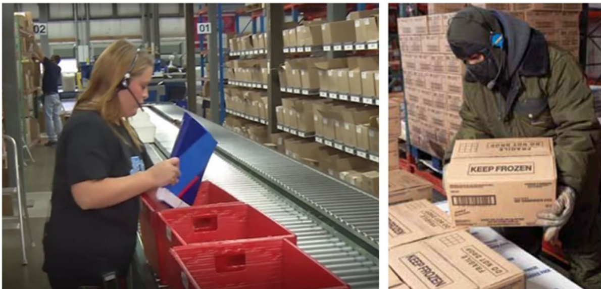
Figure 3: A worker wearing a voice unit in a distribution center placing products (brochures and pamphlets) into a train of totes (left panel); a worker in protective clothing working, order selecting in a frozen distribution center. It should be noted that the headset and the microphone worn by both workers are both wireless.
