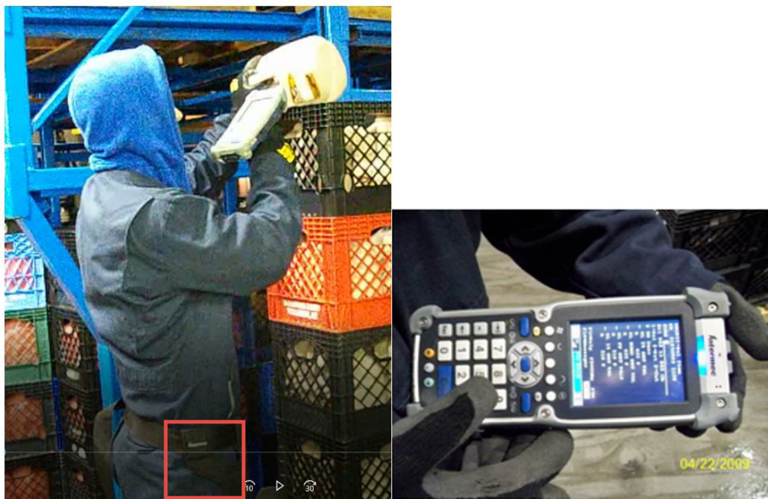
Figure 2: The order selector lifts the product in order to scan the barcoded UPC of the product (left panel). This product validity check is to confirm the product is part of the store order. Once the UPC scan is successfully completed, the user enters the number of units of the ordered product (right panel) and then holsters (left panel, red square) the device in order to select the units onto the pallet (or tote). In the right panel, the user is wearing gloves while pressing the keys on the wireless handheld device.
