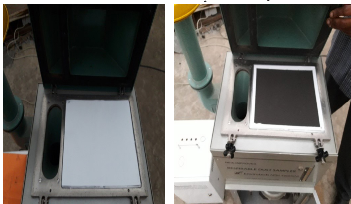
Figure 6: Before and after experiment of PM 10 sampling filter paper
