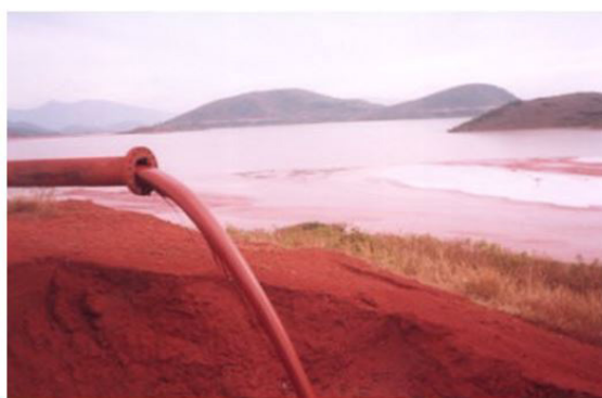
Figure 5: The pond of NALCO factory in Damandjodi (India) depicting red mud slurry disposal [26]
