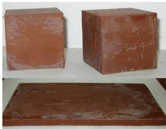
Figure 6: Geopolymers made using red mud [29]
