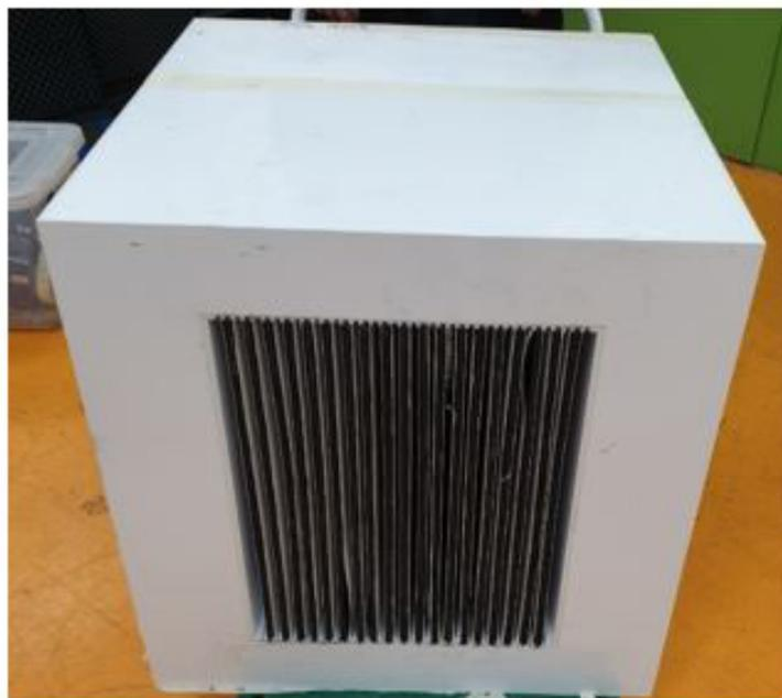
**Figure 1:** The test equipment used to minimize pressure loss for the filter efficiency measurements
