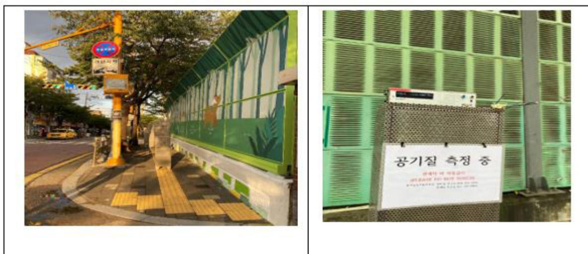
**Figure 5:** Measurement of the fine PM reduction efficiency of a Cerebasel filter in Bucheon City
