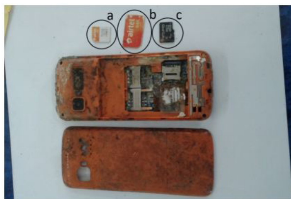
Figure 7: Cell Phone Found Inside One Pocket of the Hanging Pant Showing Dual Sim Cards (a, b) and Memory Card (c)
