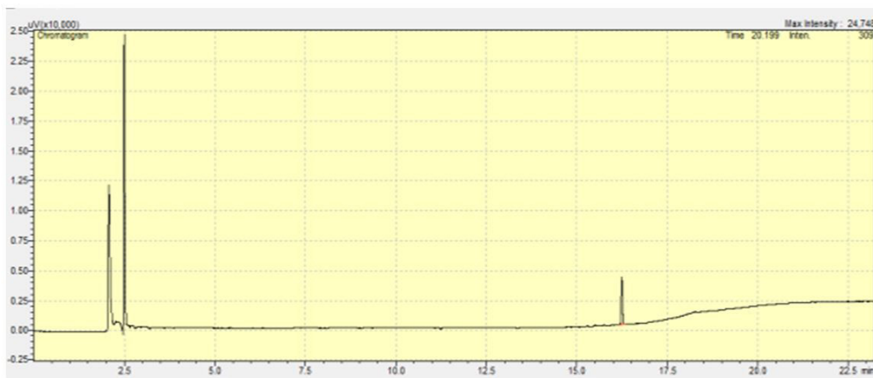
Figure 2: Gas Chromatography Chromatogram of (150ppb) Chlorpyrifos Standard
