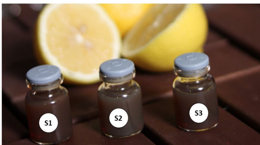
Figure 2: Silver nanoparticle prepared by adding 200 ml of silver nitrate in three different molar ratios; (S1) (3 mM), (S2) (4 mM), and (S3) (5 mM) to 40 mL lemon extract.
