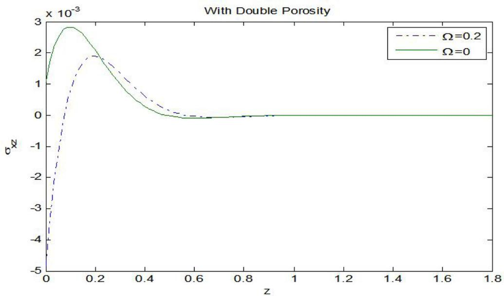
Figure 9: Distribution of the stress component  $\sigma_{xz}$
