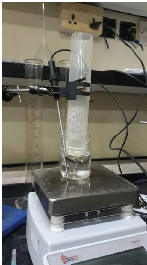
Photo 2: Locally fabricated Franz-diffusion cell; Two side open ended test tube as donor compartment in which lower opening consist of dialysis membrane as semi-permeable membrane tightened by cotton thread. Receptor compartment was filled with 60 ml phosphate buffer of pH 6.8 placed on magnetic stirrer hot plate with temperature of 37\pm 2 °C with the 100-rpm magnetic stirrer.
