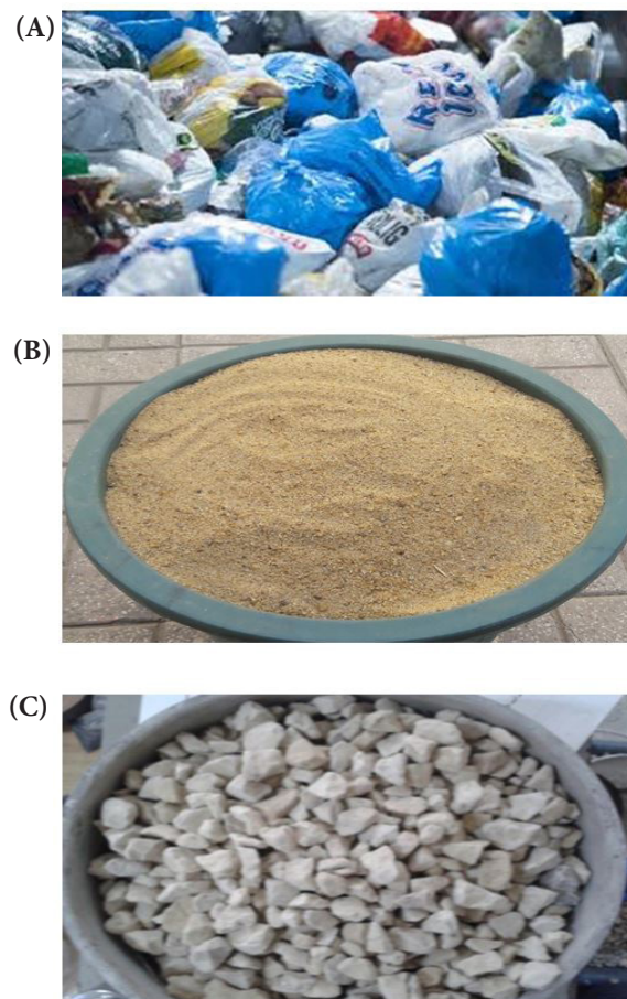
Figure 2: The materials used in the study (A) Waste plastic; (B) Sand; (C) Gravels
