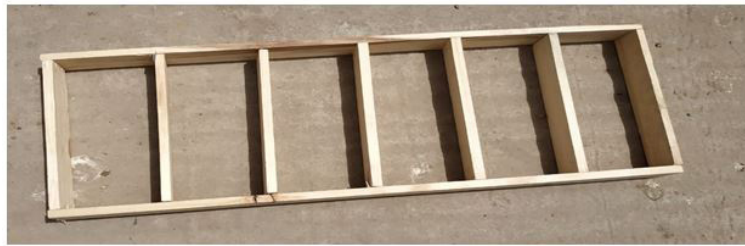
Figure 3: The mold used to form the bricks and blocks
