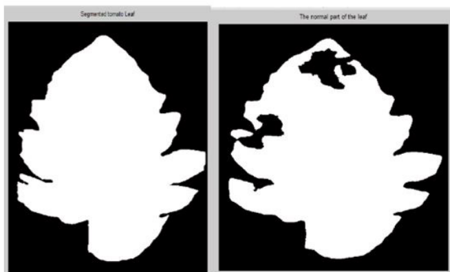
Figure 7: Extraction of normal tomato leaf area to estimate the disease severity of the leaf
