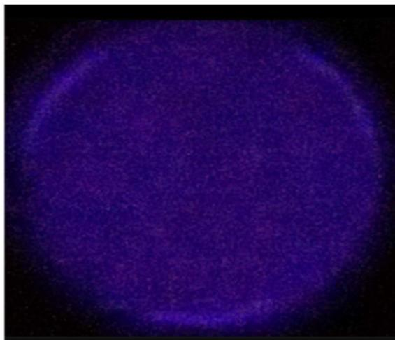
**Figure 3:** Excitation of homogeneous diffuse discharges.
