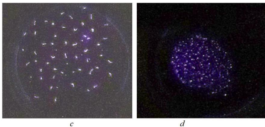
**Figure 2:** The effect of increasing the density of filamentary discharges over time with a decrease in the area of filaments occurrence. Partial conversion to diffuse discharge at cleaned copper electrode surface (b).
