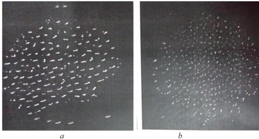
**Figure 1:** The effect of increasing the density of filamentary discharges over time without changing the area of occurrence of filaments at non-cleaned copper electrode surface.
