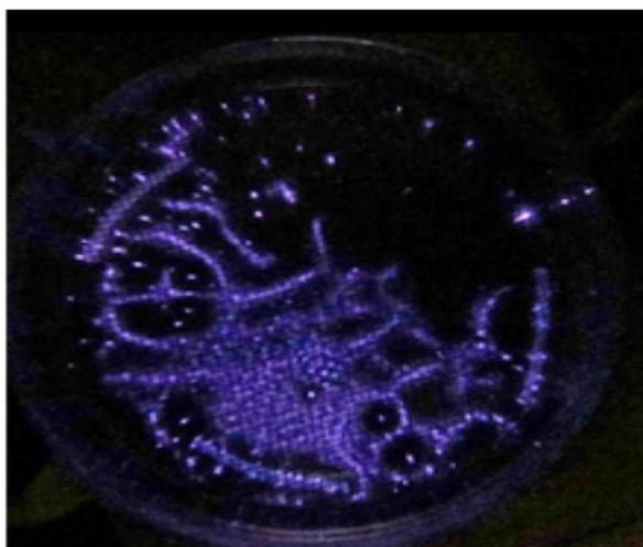
**Figure 4:** Formation of self-organized structures (case of using a reactor with two dielectrics).
