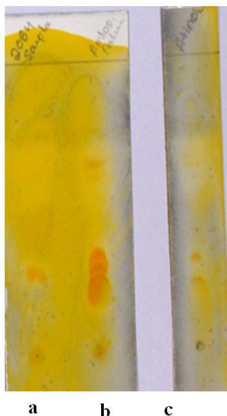
Figure 4: Visibility of orange coloured spot when sprayed with Dragandroff reagent; a: Blood Sample; b: Visceral Sample; c: Standard Atenolol
