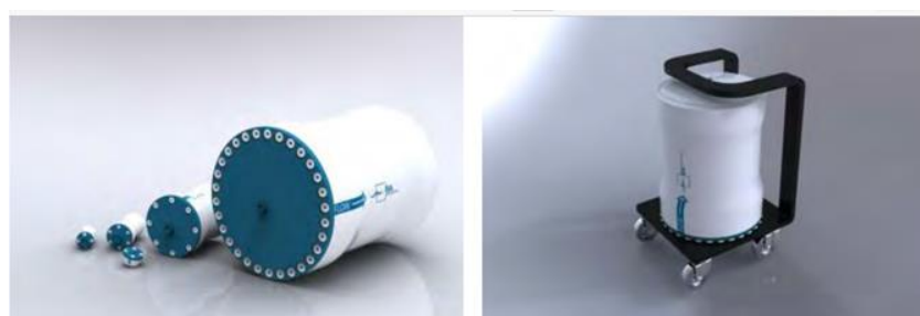
CIMmultus™ from BIA Separations (1 mL – 8 L) Carbon fibre reinforcement embedded into epoxy thermoset resin (carbon fibre composite); tough, light material; 5-times lower density than stainless-steel; operate at 20 bar (291 psi).
