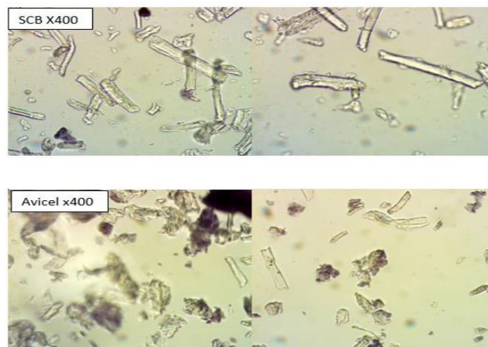
Figure 2: Light microscopic images of Novicel™ (SCB x400) and Avicel® 101 (Avicel x400)
